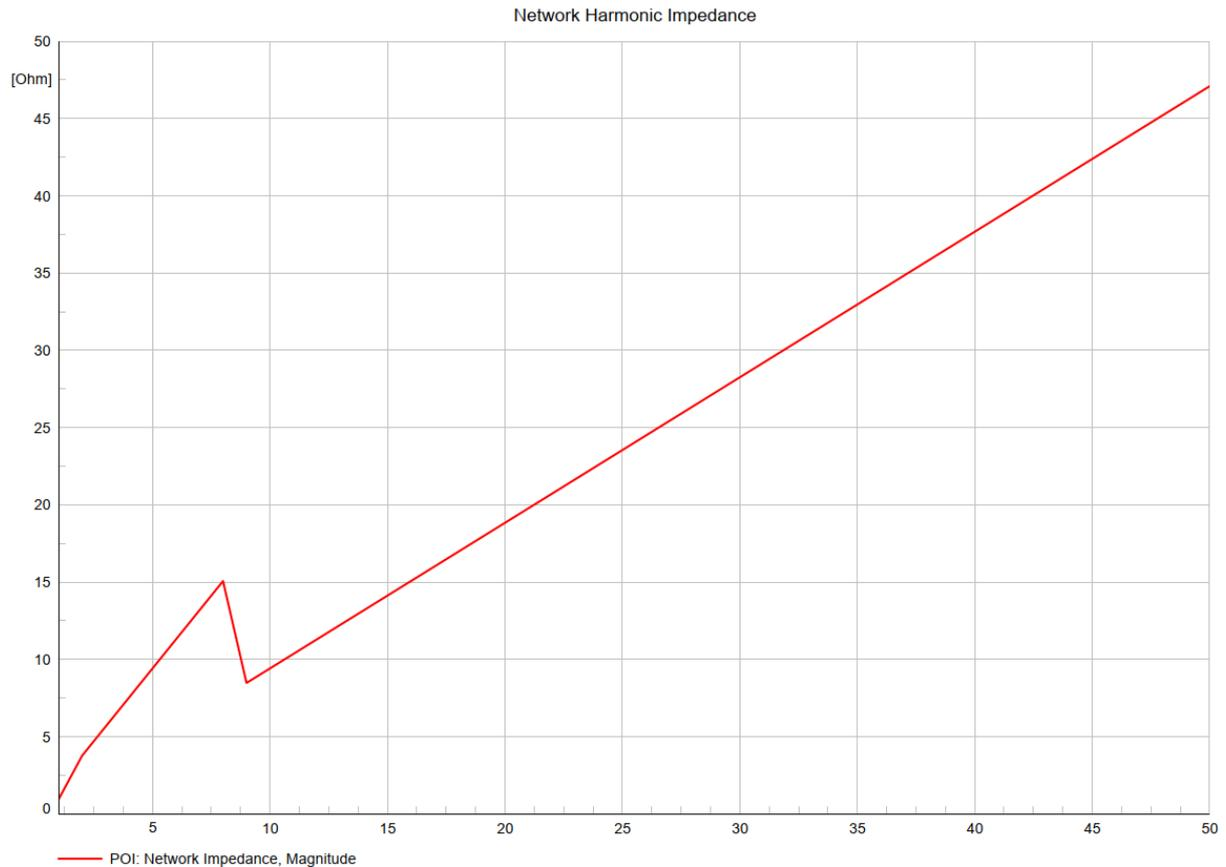
**Figure 6 – Network harmonic impedance Powerfactory model, Case 2**
