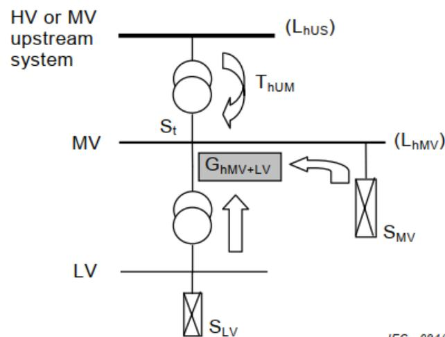
**Figure 2 – Example of a system for sharing global contributions in MV**
